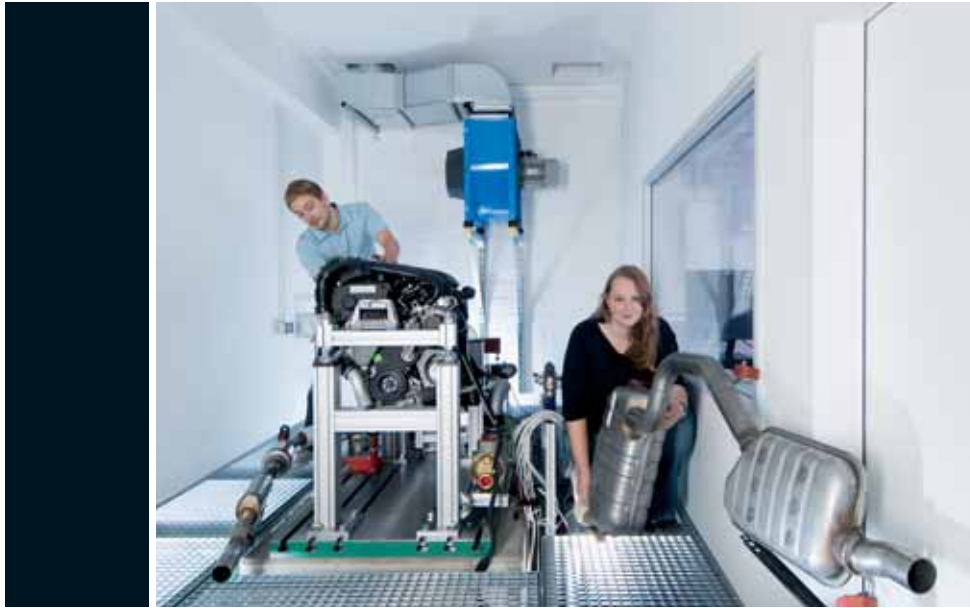
Engine test stand at the Ingolstadt facility for pre-development and qualification measures.
