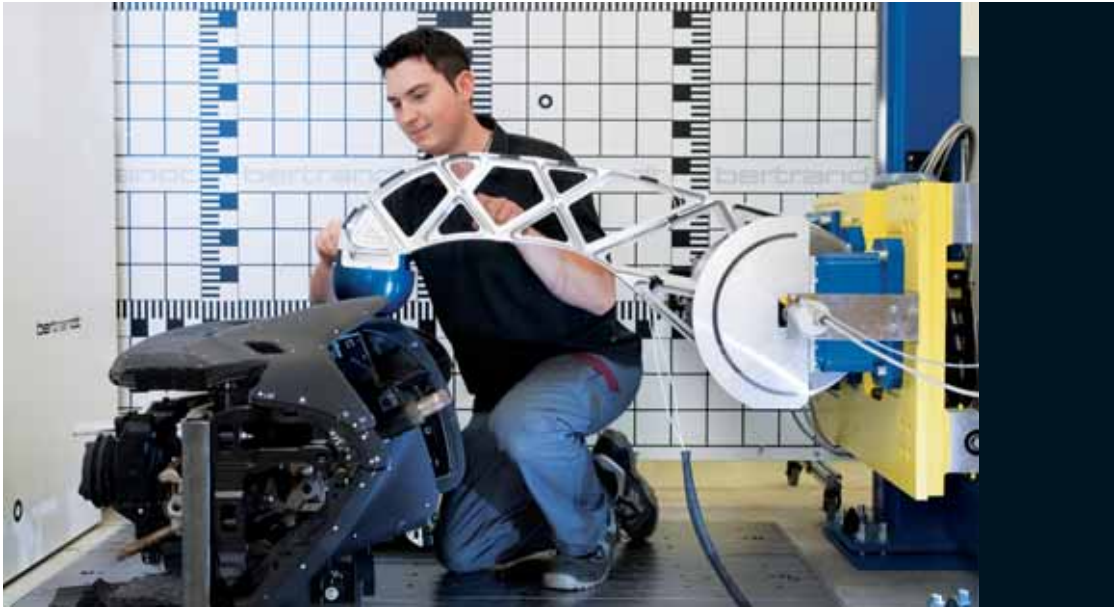
Preparation of an ECE R21 pendulum impact test
